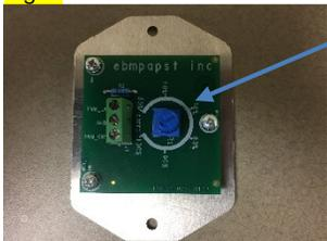
Rotate dial clockwise to increase max CFM or counter clockwise to decrease. (Used with 0-10VDC fan speed signal)
