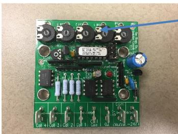
Rotate dial(s) clockwise to increase max CFM or counter clockwise to decrease. Call 1, 2 & 3 are used with 3 spd fan thermostat. (Call 4 not used) No call must be at zero flow
