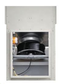
The **ACE** uses state-of-the-art 48 VDC fans to cool and ventilate telecom enclosures by drawing in outside air with fan modulation for precise flatline temperature control. The positive pressure design prevents dust and dirt infiltration.
