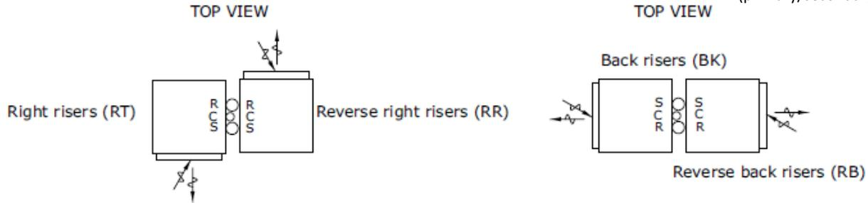
Risers are always sized based on the floor to floor height to ensure the proper assembly. To ensure proper alignment, the top of the riser should always be positioned at a distance of 92" from the floor. This distance allows all risers to be properly sized based on the distance of  $L = F + 2"$ , where the extra 2" allows for the riser to protrude to the floor below for connection.
