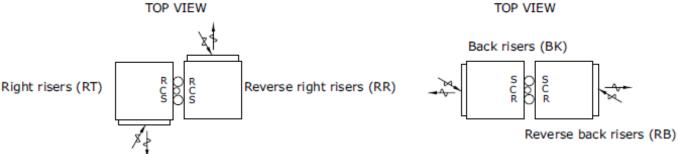
Risers are always sized based on the floor to floor height to ensure the proper assembly. To ensure proper alignment, the top of the riser is should always be positioned at a distance of 92" from the floor. This distance allows all risers to be properly sized based on the distance of L = F + 2", where the extra 2" allows for the riser to protrude to the floor below for connection.
