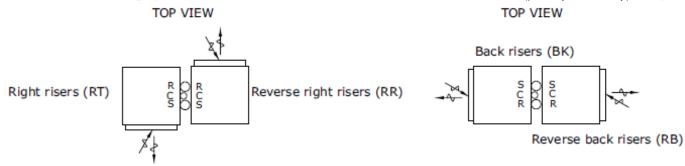
Risers are always sized based on the floor to floor height to ensure the proper assembly. To ensure proper alignment, the top of the riser is should always be positioned at a distance of 92" from the floor. This distance allows all risers to be properly sized based on the distance of L = F + 2", where the extra 2" allows for the riser to protrude to the floor below for connection.
