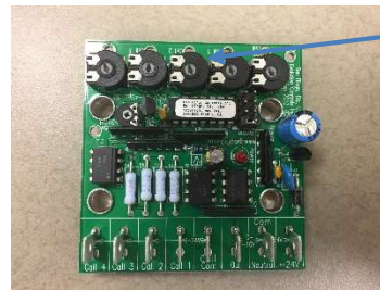
Figure 2: EVO 4-Spd CFM Adjustment Board
