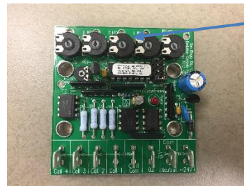
Figure 2: EVO 4-Spd CFM Adjustment Board
