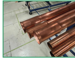
Swagged end of Risers
